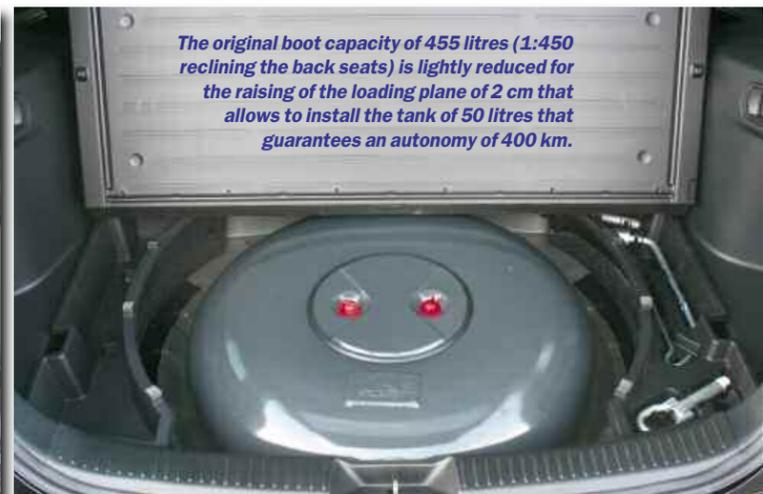
*The original boot capacity of 455 litres (1:450 reclining the back seats) is lightly reduced for the raising of the loading plane of 2 cm that allows to install the tank of 50 litres that guarantees an autonomy of 400 km.*
