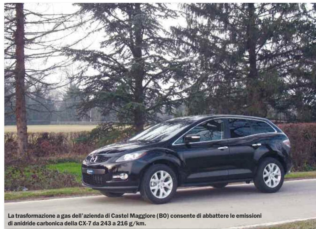
*The gas transformation of the company of Castel Maggiore (BO) allows to decrease the carbon dioxide emissions of the CX-7 from 243 to 216 g/km.*
