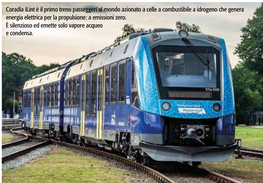
Coradia iLint is the first passenger train in the world powered by hydrogen fuel cells that generates electricity for propulsion: with zero emissions. It is silent and emits only water vapor and condensation.
