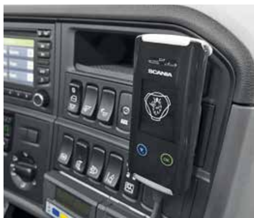
Alcolock Scania installed on the dashboard.
