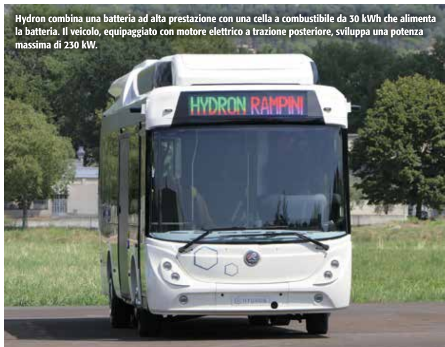
Hydron combines a high performance battery with a 30 kWh fuel cell. The vehicle, equipped with a rear-wheel drive electric motor, develops a maximum power of 230 kW.
