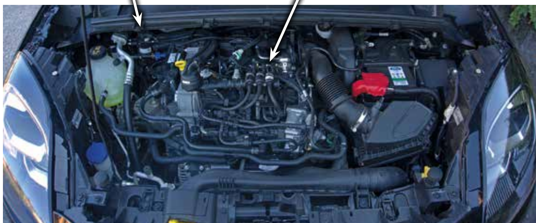
The 3-cylinder 1.0 EcoBoost is supported by the electric motor for a total of 125 HP. The power remained unchanged applying the Sequent Maestro kit.
