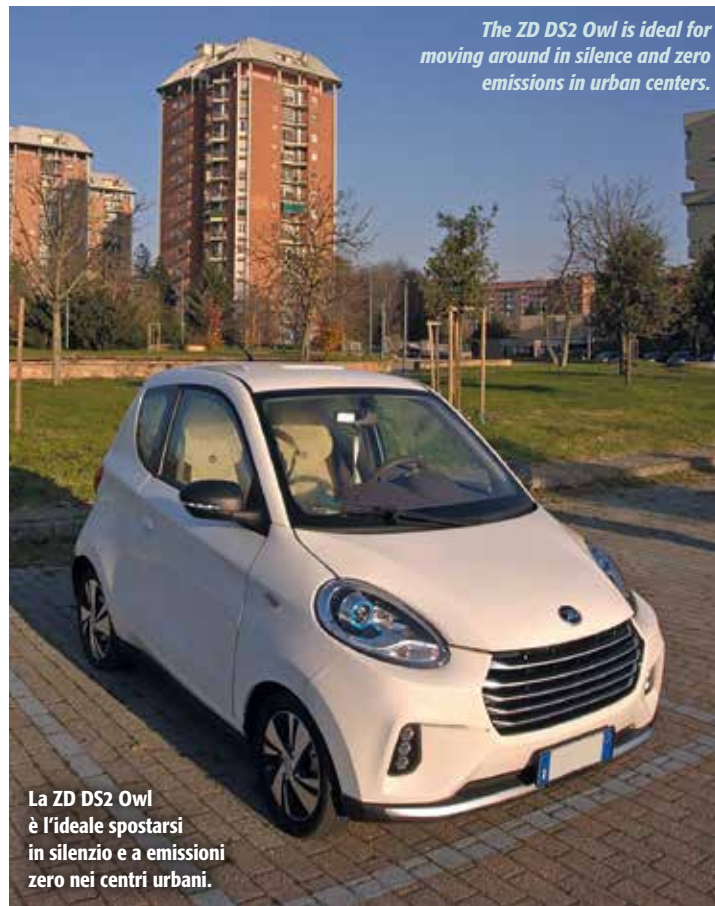
The DS2 has 27 kWh batteries for urban ranges up to 280 km.
