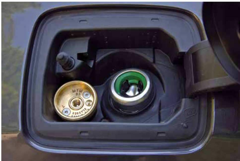
The gas filling socket with the adapter is inside the petrol refueling flap.
