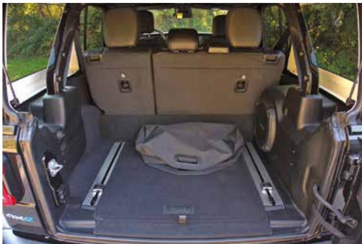
The batteries under the back seats leave unmodified the 533 l trunk capacity, 1,910 l if the back seats are fully reclined.
