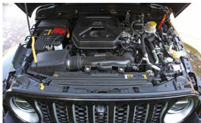
To the 2.0 turbo with 272 HP, there are two additional electric engines for an overall 380 HP and 673 Nm.
