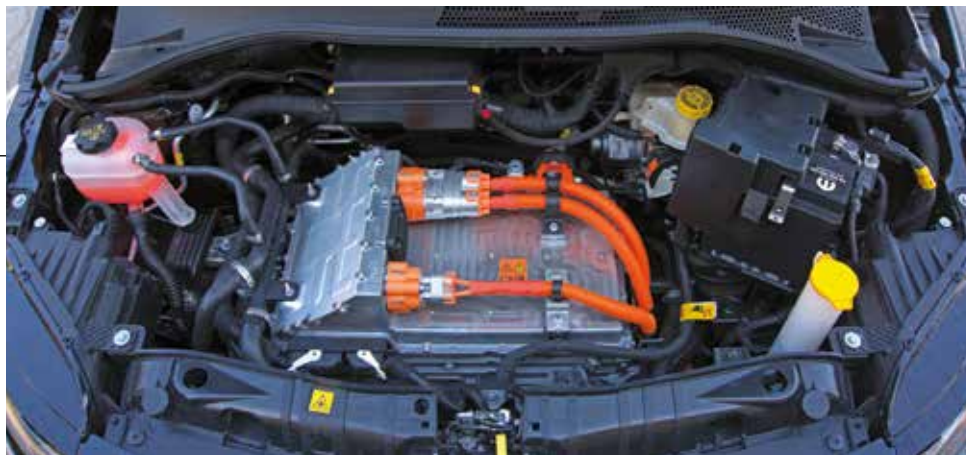
The entire electrical system (excluding batteries) is enclosed under the hood, including, among other things, a three-phase permanent magnet synchronous motor, inverter and AC-DC converter.
