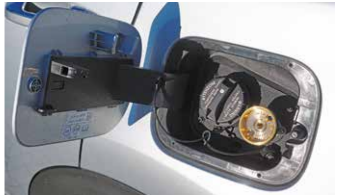
The gas filling inlet is inside the hatch for petrol inlet.
