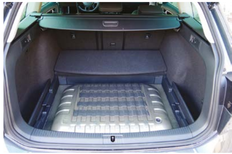
The Variant has a well detailed trunk that can hold up to 424 l. It can hold up to 1,439 l by flattening the back seats. The 15 kg gas tanks are under the loading plan.
