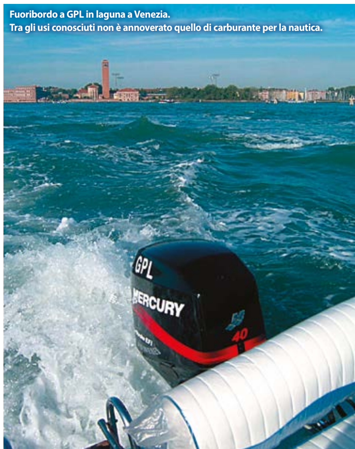
LPG fueled overboard in the Venice Lagoon. One of the lesser known uses of LPG is for boating.
